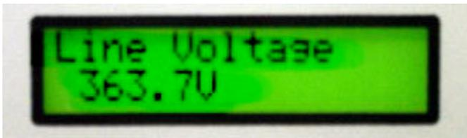
*Monitor the values of line and load voltages, currents, etc using true RMS measurements.*
