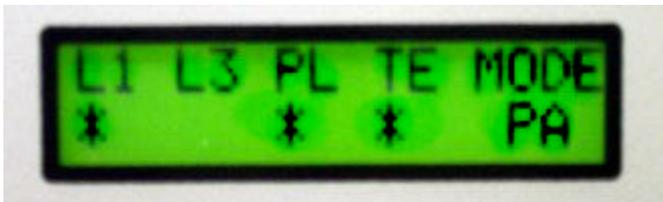
*Monitor the stack operating status either on the display or using communications. (The illustration shows line 1 present, that the stack is phase locked, that the heatsink temperature is OK and the firing mode is phase angle).*
